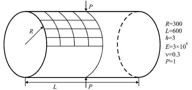
Shell of revolution with geometrical parameters:
