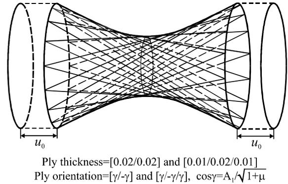
Fig. 8. Angle-ply hyperbolic shell subjected to uniform stretching.
