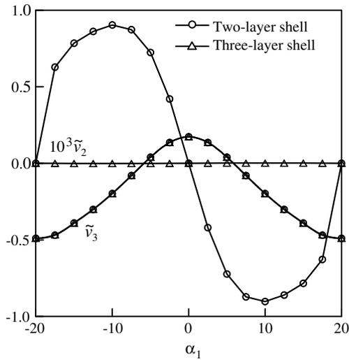
Fig. 9. Circumferential and transverse displacements of middle surface  $\tilde{v}_{\alpha+1} = v_{\alpha+1}^M/u_0$  of hyperbolic shell versus coordinate  $\alpha_1$ .
