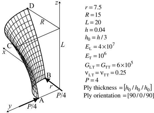
Shell of revolution with geometrical parameters:
