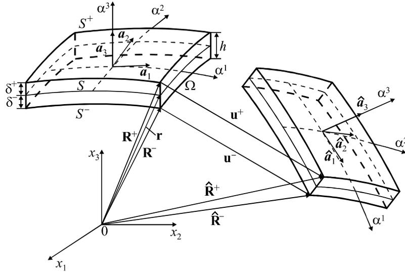
Fig. 2. Geometry and kinematics of shell.
