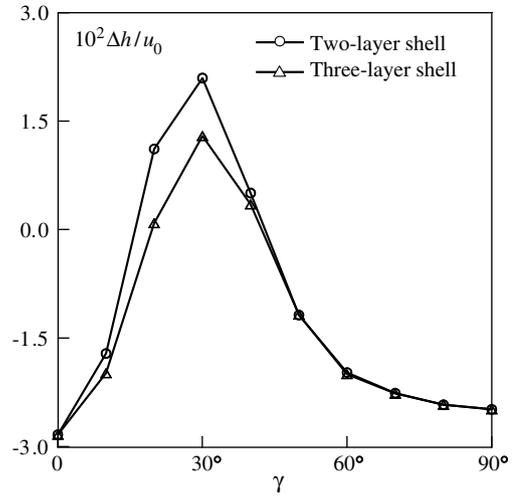
Fig. 6. Thickness change  $\Delta h = v_3^+ - v_3^-$  at central section of cylindrical shell versus ply angle  $\gamma$ .
