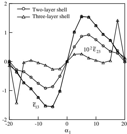
Fig. 10. Transverse shear strains of middle surface  $\tilde{\epsilon}_{\alpha 3} = 50L\epsilon_{\alpha 3}^M/u_0$  of hyperbolic shell versus coordinate  $\alpha_1$ .
