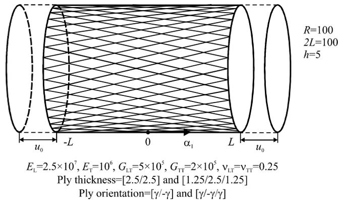
Fig. 5. Angle-ply cylindrical shell subjected to uniform stretching.
