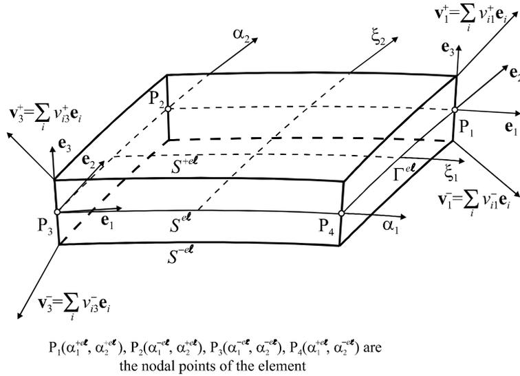
Fig. 3. Four-node geometrically exact solid-shell element.
