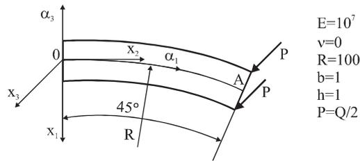
Fig. 14. Cantilever curved beam under tip couple forces.
