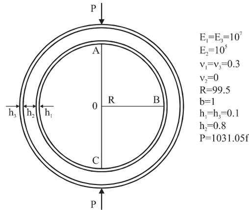
Fig. 12. Pinched circular sandwich ring.
