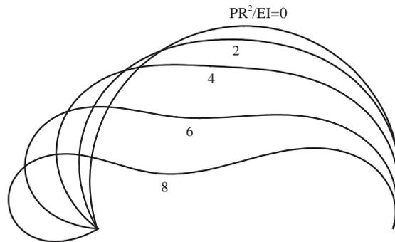
Fig. 11. Deformed configurations of deep clamped-hinged arch under apex load.
