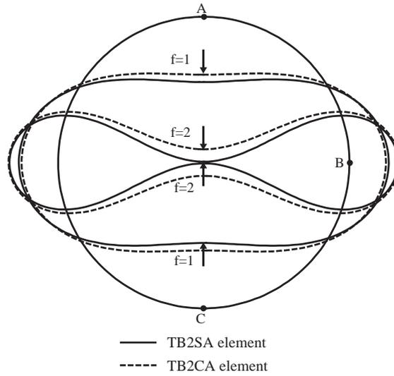
Fig. 13. Deformed configurations of pinched circular sandwich ring.
