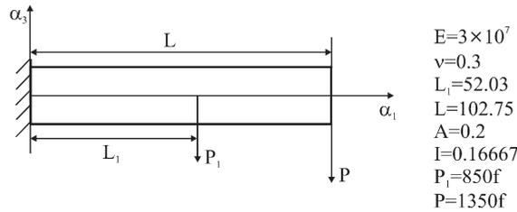
Fig. 8. Cantilever beam under two transverse loads.
