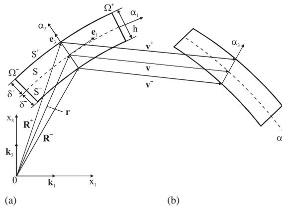
Fig. 1. Curved beam: (a) initial configuration and (b) final configuration.
