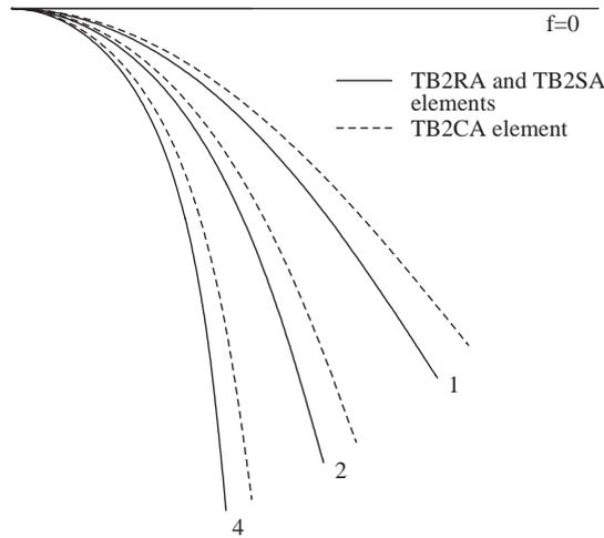
Fig. 9. Deformed configurations of cantilever beam under two transverse loads.
