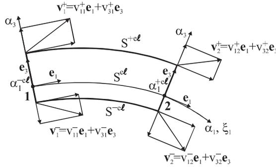
Fig. 4. Two-node curved beam element.
