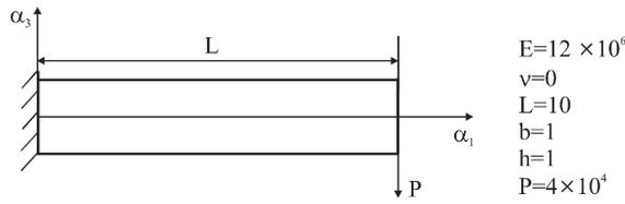
Fig. 6. Cantilever beam under shear tip load.
