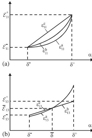
Fig. 2. Distribution of (a) longitudinal strain and (b) transverse shear strain over beam thickness.
