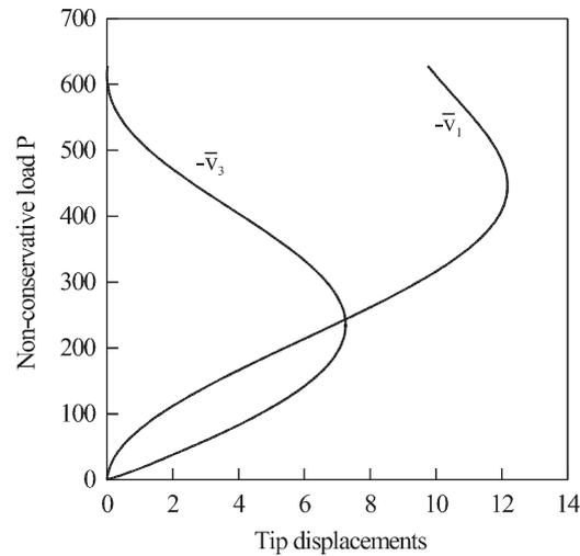
Fig. 16. Longitudinal and transverse tip displacements  $\bar{v}_i = (v_i^- + v_i^+)/2$  of cantilever beam under non-conservative couple forces.
