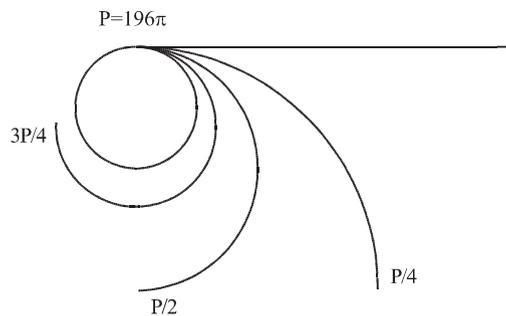
Fig. 17. Deformed configurations of cantilever beam under non-conservative couple forces.
