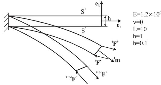
Fig. 15. Deformed configurations of cantilever beam under non-conservative couple forces.
