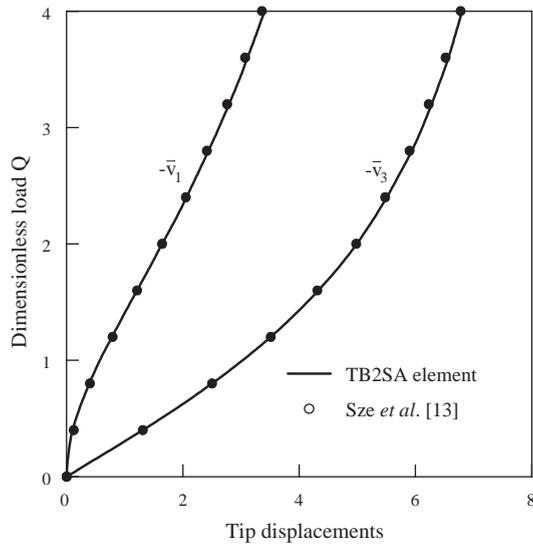
Fig. 7. Longitudinal and transverse tip displacements  $\bar{v}_i = (v_i^- + v_i^+)/2$  of cantilever beam under shear tip load.
