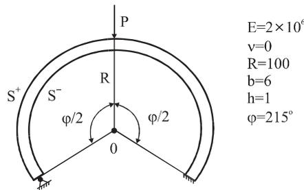
Fig. 10. Deep clamped-hinged arch under apex load.
