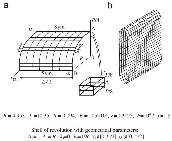
Fig. 16. Pulled cylindrical shell: (a) geometry and (b) deformed configuration for  $f = 1.95$  (modeled by  $8 \times 12$  mesh).
