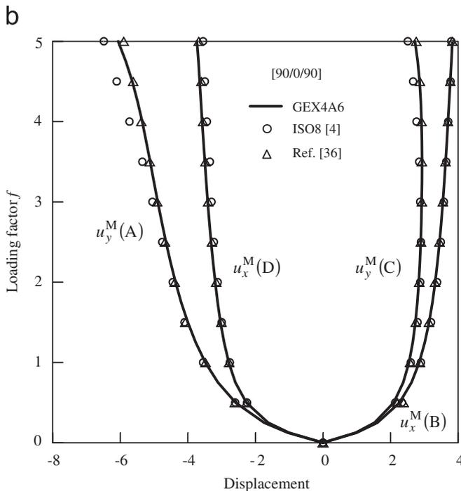
Fig. 21. Midsurface displacements of pinched cross-ply hyperbolic shell for ply orientations: (a) [0/90/0] and (b) [90/0/90] (modeled by  $28 \times 28$  mesh).
