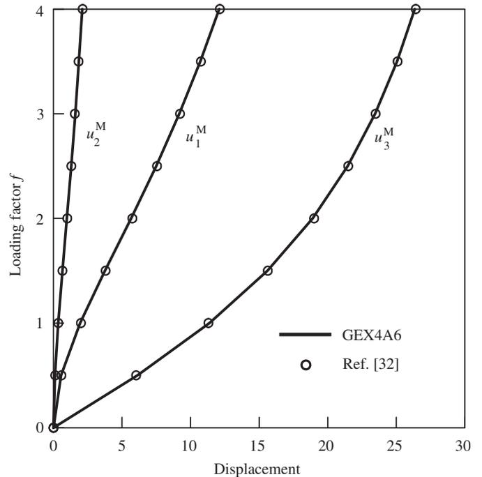
Fig. 7. Midplane displacements under applied loads of cantilever plate (modeled by  $8 \times 6$  mesh).
