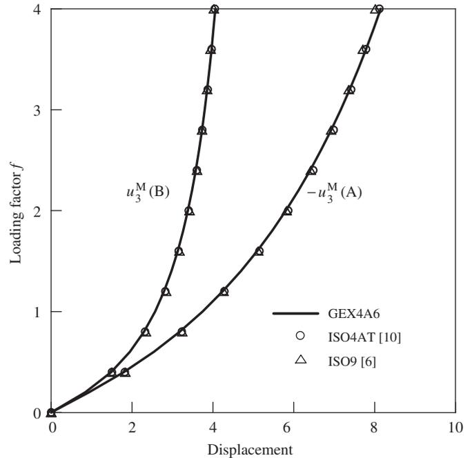
Fig. 10. Midsurface displacements of pinched hemispherical shell (modeled by  $16 \times 16$  mesh).
