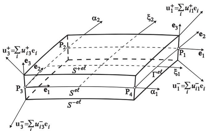
$P_1(\alpha_1^{+el}, \alpha_2^{+el}), P_2(\alpha_1^{-el}, \alpha_2^{+el}), P_3(\alpha_1^{-el}, \alpha_2^{-el}), P_4(\alpha_1^{+el}, \alpha_2^{-el})$  are the nodal points of the element
