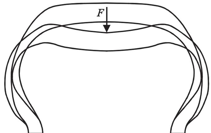
Fig. 24. Deformed tire section.
