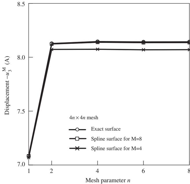
Fig. 12. Convergence study due to mesh refinement for pinched hemispherical shell with GEX4A6 element.
