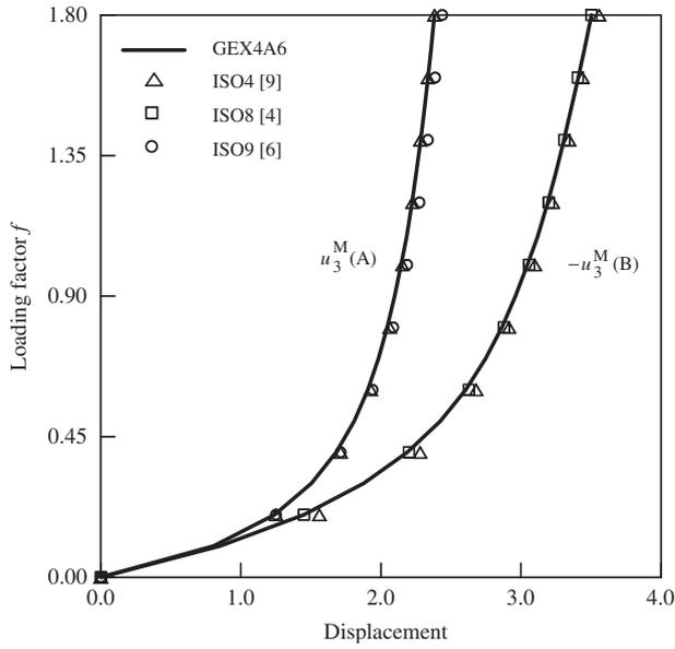
Fig. 18. Midsurface displacements of pulled cylindrical shell (modeled by  $8 \times 16$  mesh).
