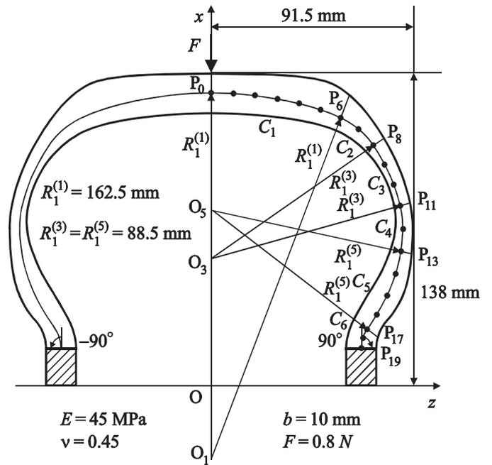
Fig. 22. Polyurethane tire section.
