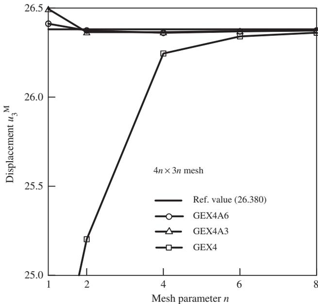
Fig. 6. Convergence study due to mesh refinement for cantilever plate, where reference solution is provided by  $64 \times 48$  mesh of GEX4A6 elements.
