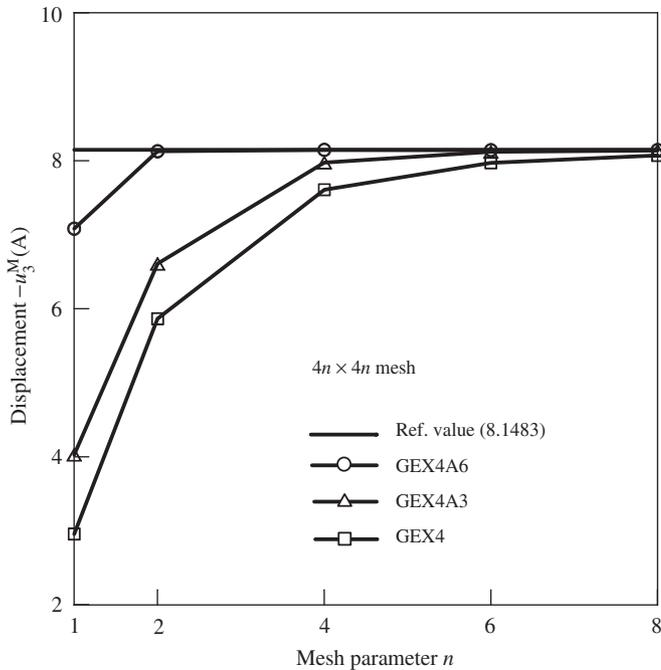
Fig. 9. Convergence study due to mesh refinement for pinched hemispherical shell, where reference solution is provided by  $64 \times 64$  mesh of GEX4A6 elements.
