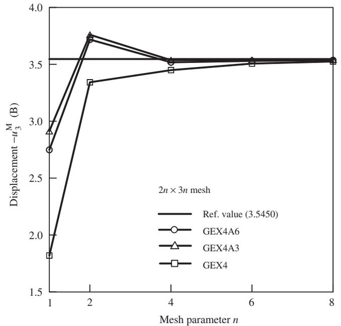
Fig. 17. Convergence study due to mesh refinement for pulled cylindrical shell, where reference solution is provided by  $32 \times 48$  mesh of GEX4A6 elements.
