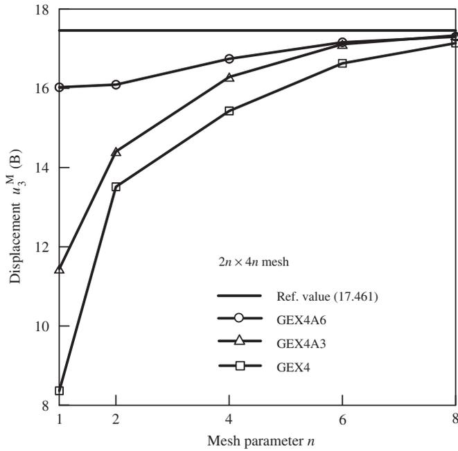
Fig. 14. Convergence study due to mesh refinement for slit ring plate, where reference solution is provided by  $32 \times 64$  mesh of GEX4A6 elements.
