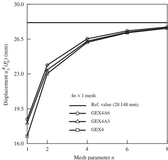
Fig. 23. Convergence study due to mesh refinement for tire section, where reference solution is provided by  $64 \times 1$  mesh of GEX4A6 elements.
