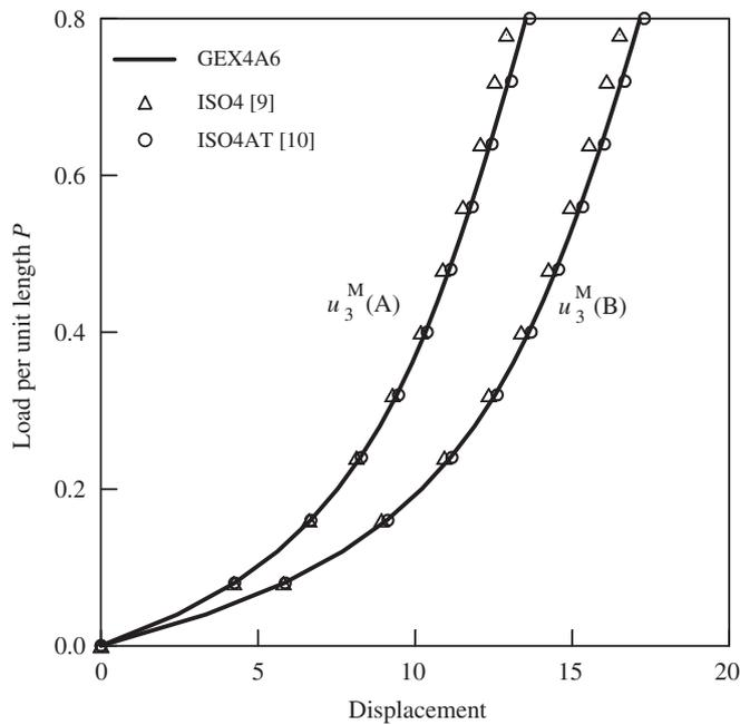
Fig. 15. Midplane displacements of slit ring plate (modeled by  $6 \times 30$  mesh).
