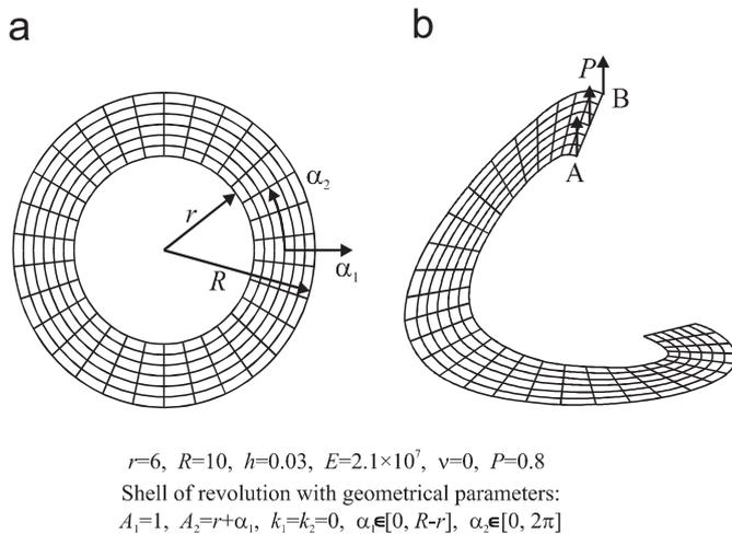
Fig. 13. Slit ring plate under line load: (a) geometry and (b) deformed configuration (modeled by  $6 \times 30$  mesh).
