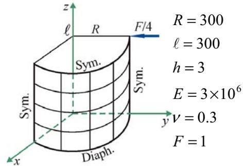
Figure 4: Pinched cylindrical shell with rigid diaphragms
