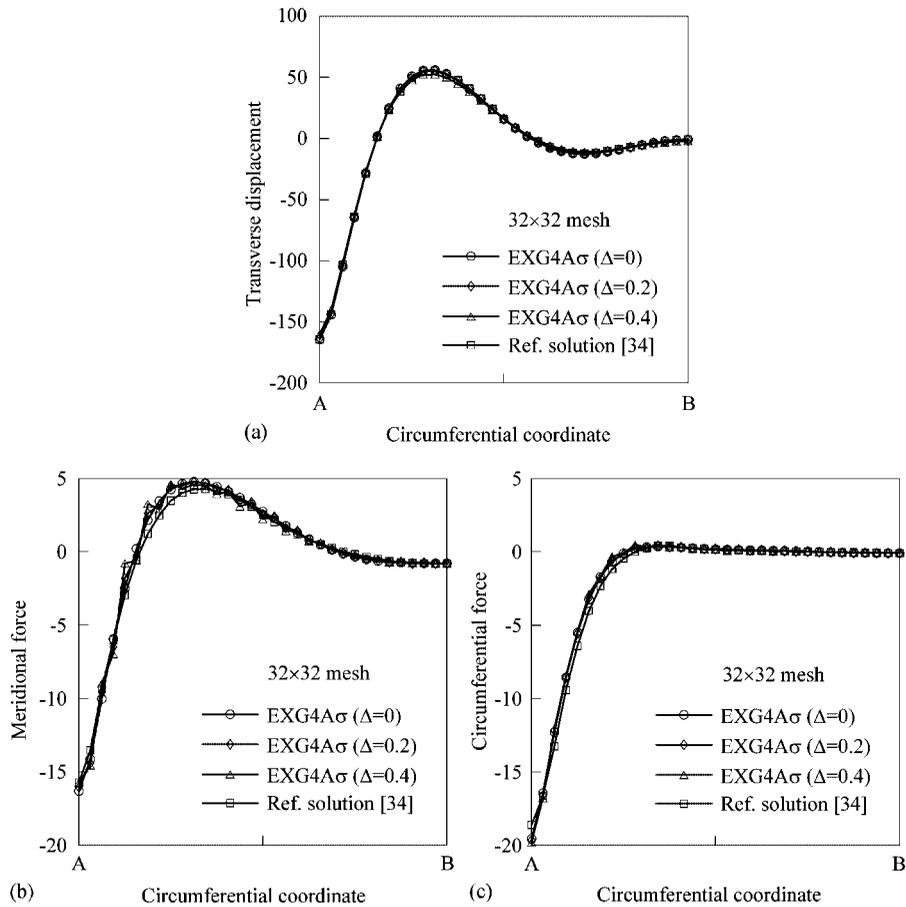
Figure 13. Results for a pinched cylindrical shell for various values of the distortion parameter: (a) transverse displacement  $Ehw/F$ , (b) meridional force  $RN_{11}/F$  and (c) circumferential force  $RN_{22}/F$ .
