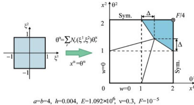
Figure 7. Simply supported square plate with a distorted  $2 \times 2$  mesh.
