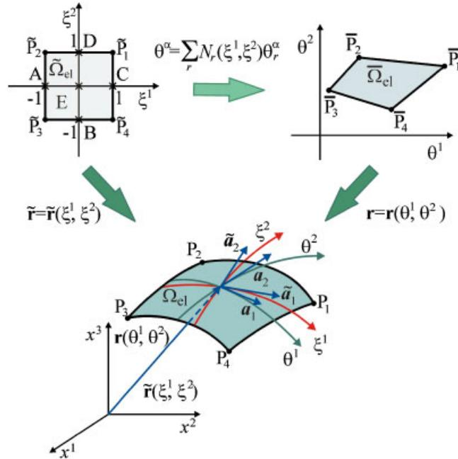
Figure 3. Biunit square in  $(\xi^1, \xi^2)$ -space mapped into the four-node exact geometry shell element in  $(x^1, x^2, x^3)$ -space.
