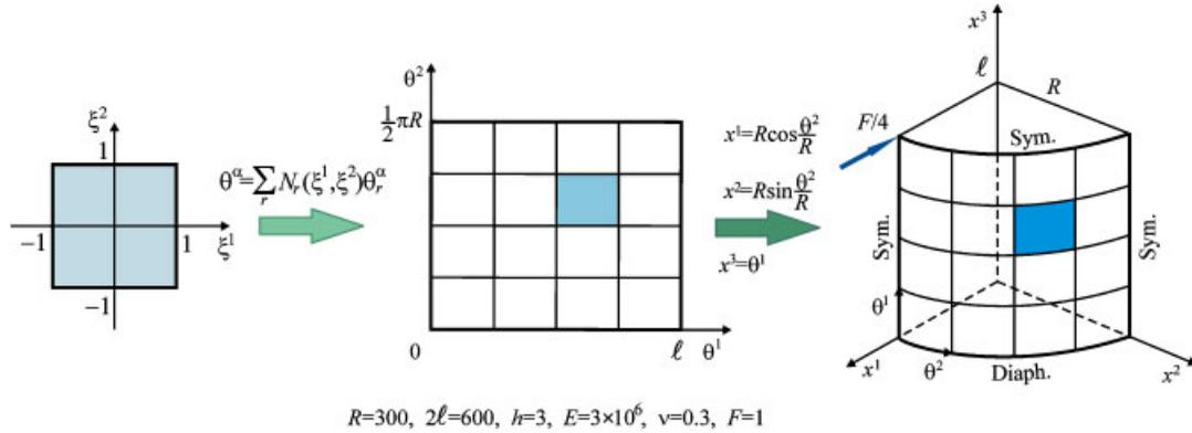
Figure 10. Pinched cylindrical shell with rigid diaphragms.
