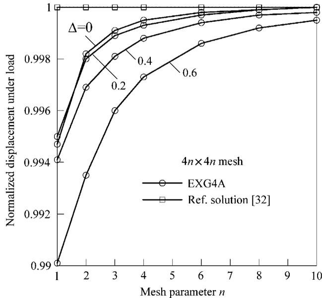
Figure 9. Convergence study due to mesh refinement and mesh distortion for a simply supported square plate.
