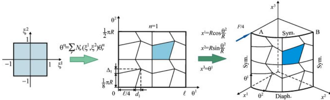
Figure 11. Pinched cylindrical shell with distorted  $4n \times 4n$  meshes, where the distortion parameters  $d_n = \ell \Delta / 4n$  and  $\Delta_n = \pi R \Delta / 8n$  ( $n = 1, 2, \dots, 10; \Delta \in [0, 0.5]$ ).
