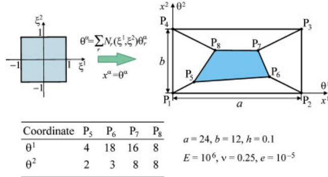
Figure 4. Plate patch test.
