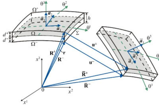
Figure 1. Initial and current configurations of the shell.
