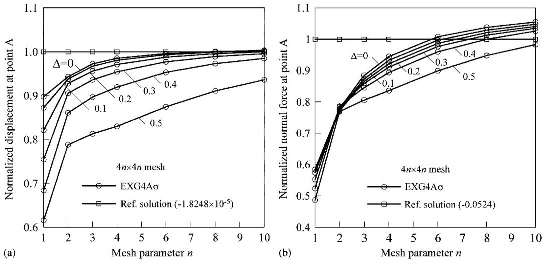
Figure 12. Convergence study due to mesh refinement and mesh distortion for a pinched cylindrical shell: (a) transverse displacement and (b) meridional force  $N_{11}$ , where the reference solution is provided by Lindberg *et al.* [34].
