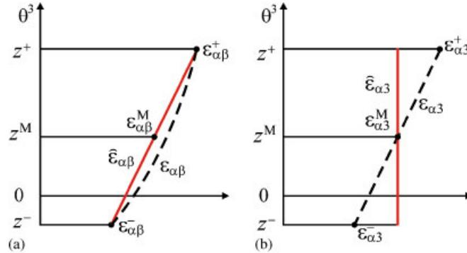
Figure 2. Approximate (—) and exact (---) distributions of: (a) in-plane and (b) transverse shear strains through the thickness of the shell.
