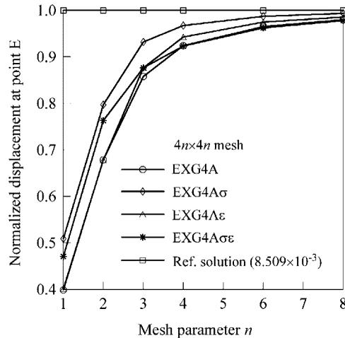
Figure 16. Convergence study due to mesh refinement for a spiral cylindrical shell, where the reference solution is provided by the  $64 \times 64$  mesh of EXG4A $\sigma$  elements.
