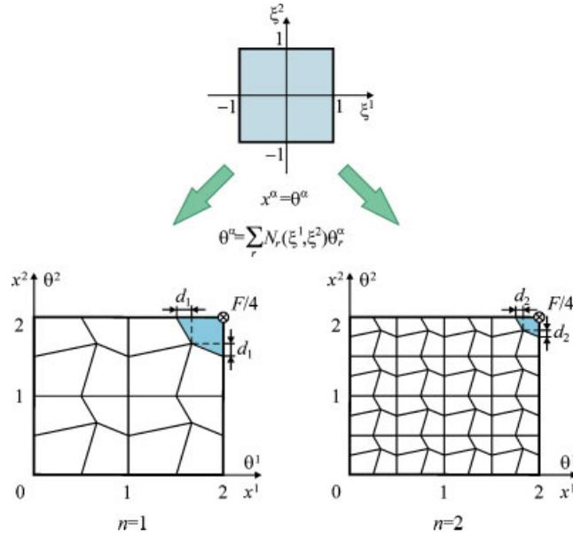
Figure 8. Simply supported square plate with distorted  $4n \times 4n$  meshes, where the distortion parameter  $d_n = \Delta/2n$  ( $n = 1, 2, \dots, 10; \Delta \in [0, 0.6]$ ).
