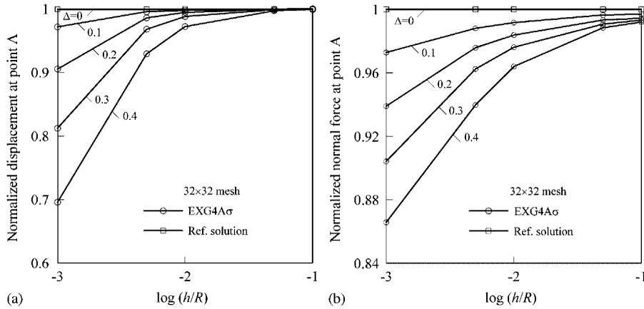
Figure 14. Results for a pinched cylindrical shell for various values of the slenderness ratio and the distortion parameter: (a) normalized transverse displacement and (b) normalized circumferential force  $N_{22}$ .
