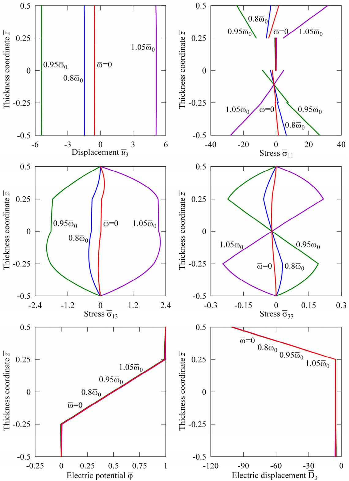
**Figure 3:** Through-thickness distributions of transverse displacement, stresses, electric potential and electric displacement for the four-layer plate subjected to electric loading (problem B)
