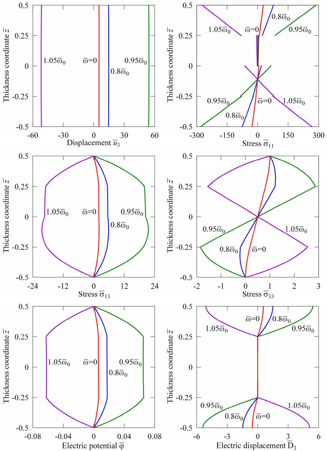
**Figure 2:** Through-thickness distributions of transverse displacement, stresses, electric potential and electric displacement for the four-layer plate subjected to mechanical loading (problem A)
