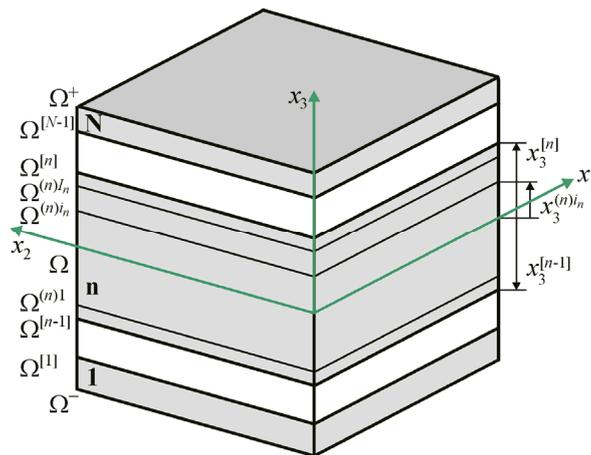
Figure 1: Geometry of the laminated piezoelectric plate
